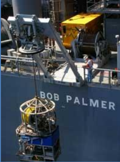
Recovery of the Nemesis ROV during subsea operations
